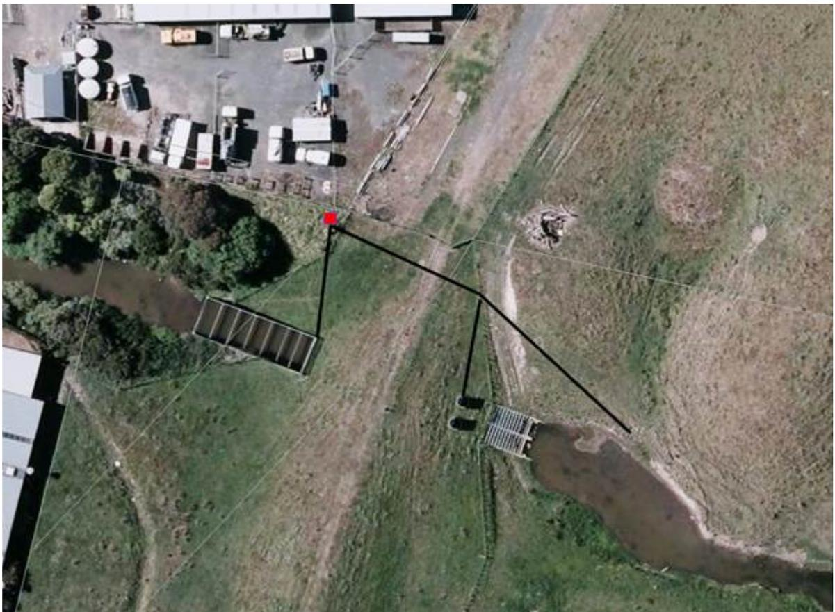
Figure 2: GIS screenshot showing the proposed location for the container (shown in red) and the trenches required to install the equipment (black lines)
