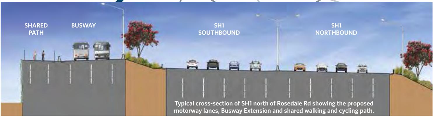
Typical cross-section of SH1 north of Rosedale Rd showing the proposed motorway lanes, Busway Extension and shared walking and cycling path.
