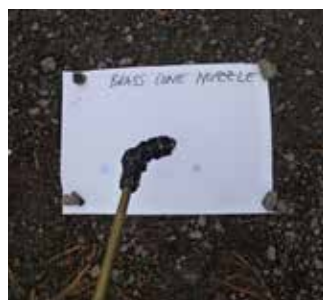
Backpack Sprayer Use a long brass wand and brass cone nozzle and anti drip filter
