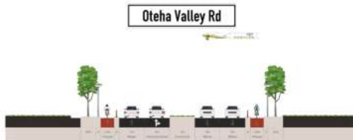
Figure 1. The space available on Oteha Valley Road can be arranged to include protected cycle lanes, while maintaining the existing traffic and pedestrian facility.
