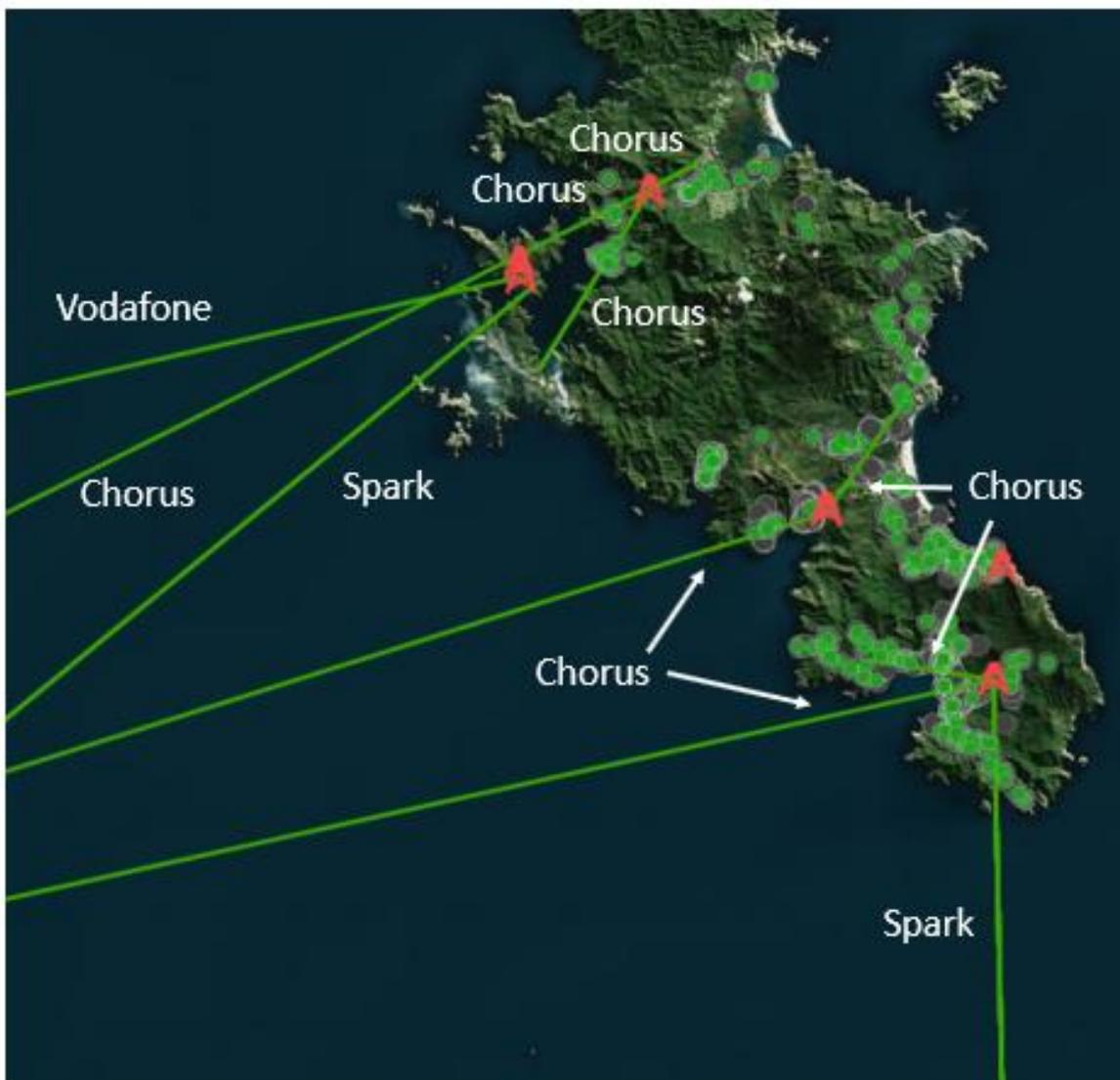
Figure 17: Microwave backhaul links running to and within Aotea Great Barrier.
