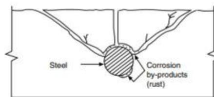
Fig 5: Tension crack due to rebar corrosion
