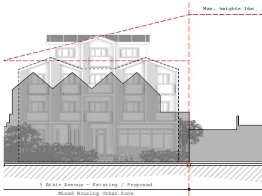
Figure 3: Identifying the existing, consented and proposed height of the building at 5 Atkin Avenue
