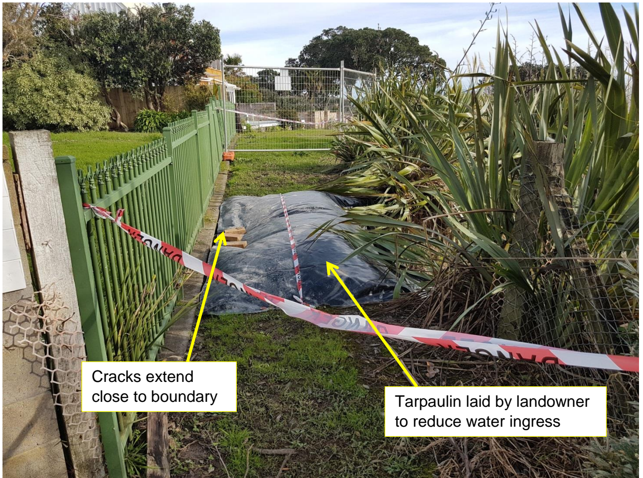
Figure 2: Photograph of landslide crest, looking west. Private property at 3 Pohutukawa Road on the left of the image.
