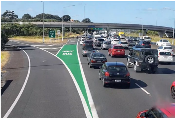
Figure 1: NX1 / NX2 buses can now continue straight into the bus only lane from the Onewa Road off ramp lane
