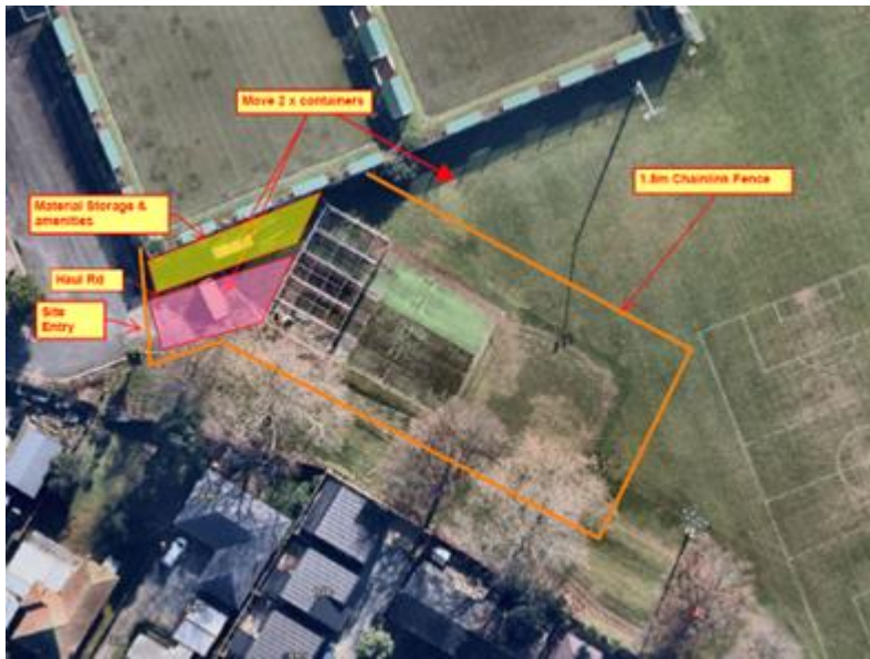
Figure 3: Aerial image showing the proposed construction area
