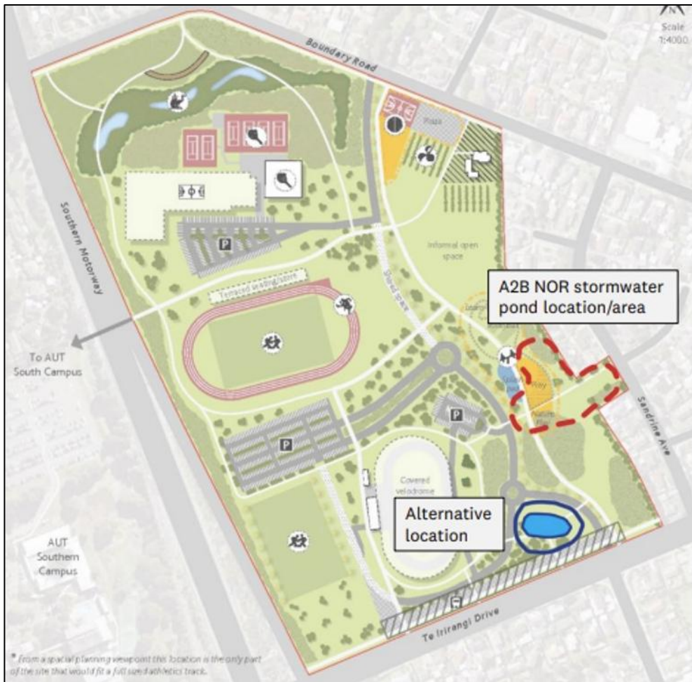
Figure 2: MSB Master Plan showing existing and recommended alternative A2B stormwater wetland location
