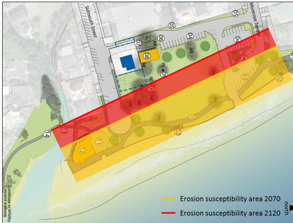
Figure 1.1: Concept plan for the Development Plan overlain with the erosion susceptibility area for the next 50 and 100 years (adapted from WSP Opus, 2018)
