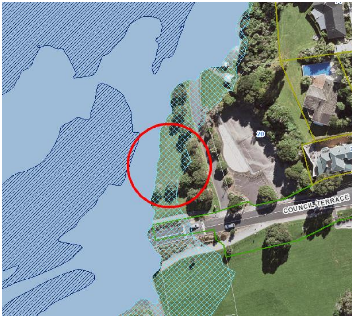
Figure 3. Proposed terrain location and flood plain (solid blue) and flood sensitive area (light blue crosshatched).
